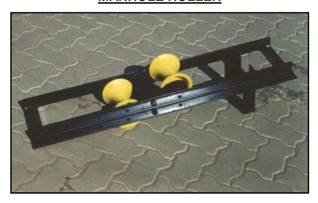
Manhole rollers are used to ease tension of cable pulling operations by reducing the drag created when pulling cable into ducts or manholes. The frame is fitted with double swinging rollers to allow the cable or rope to find its natural path. Rollers are available in polyurethane and alluminium. Manhole rollers are manufactured on order only. A standard lead time of 2-3 weeks from receipt of order is applicable subject to quantities and roller selection.
